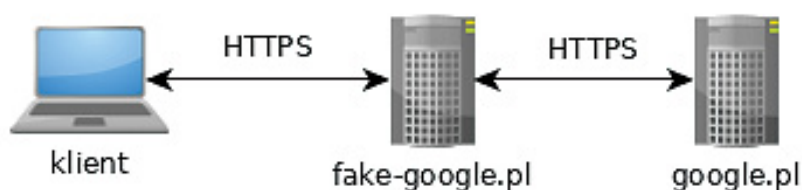
Figure 67. Diagram illustrating a reverse proxy attack.
